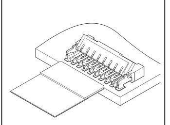
This FXVL connector is a space saving and low profile connector for FPC demanded from the market, and realizes 0.3 mm pitch connector with a mounting height of 0.9 mm and depth of 2.68 mm. In 0.3 mm pitch FPC connector, the smallest product in mounting area on the board has been provided.
